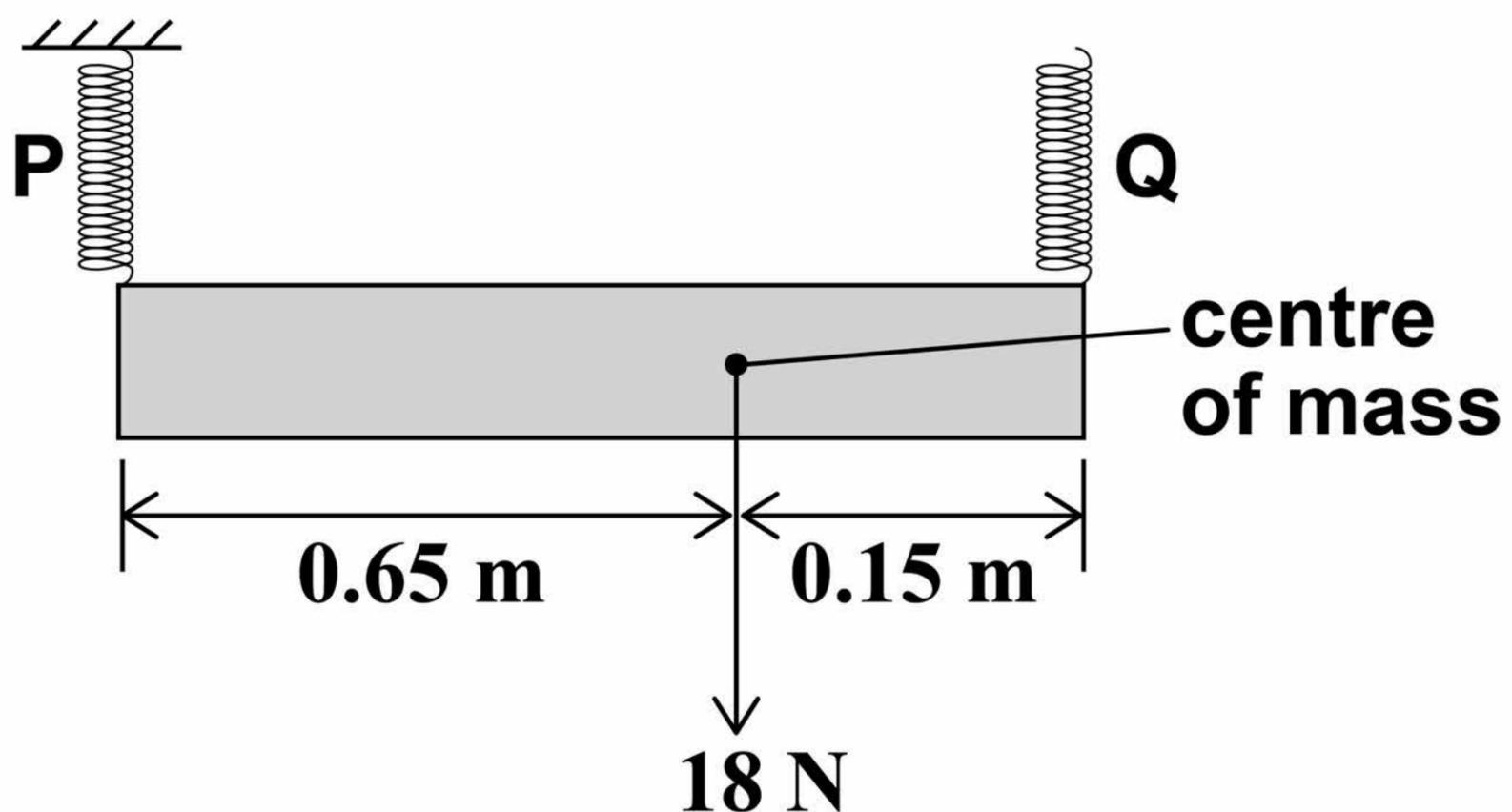
The top end of spring P is fixed and the top end of spring Q is adjusted until the sign is horizontal and in equilibrium.
