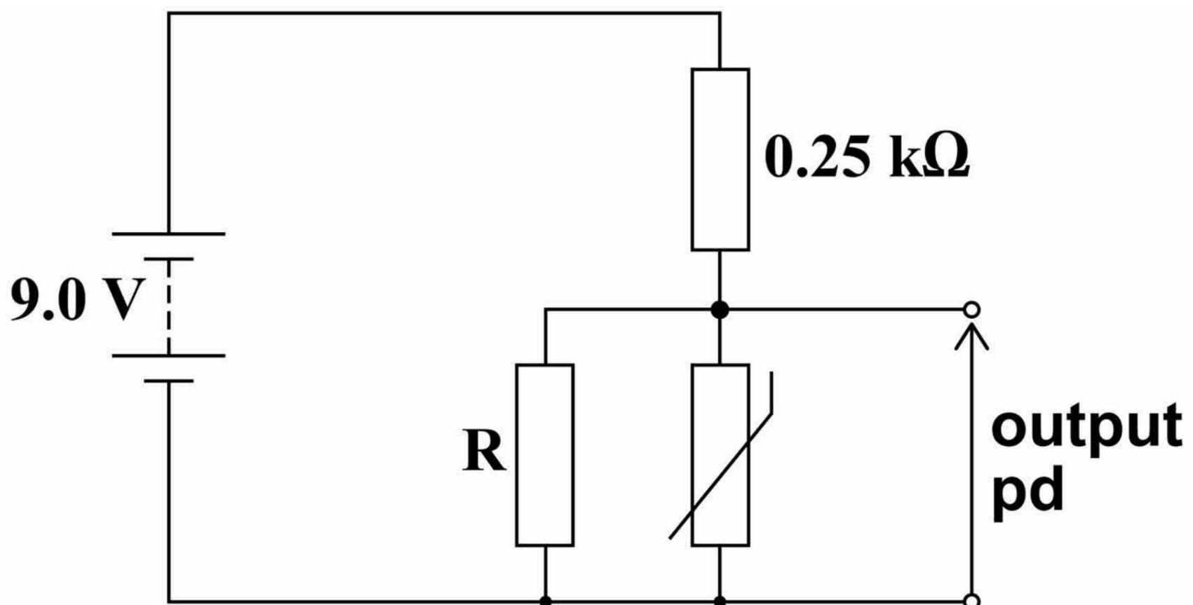
The supply has negligible internal resistance and the thermistor has a resistance of  $750 \Omega$  at room temperature. The student wants the output potential difference (pd) at room temperature to be  $5.0 \text{ V}$
