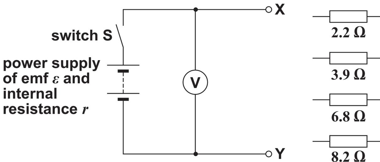
The student can change the external resistance  $R$  of the circuit between terminals  $X$  and  $Y$ . This is done by connecting different combinations of TWO resistors in series or in parallel between  $X$  and  $Y$ . This method can produce 12 DIFFERENT VALUES for  $R$ .
