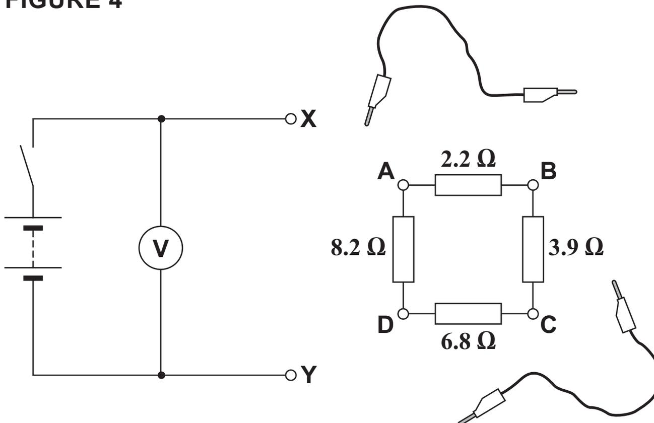
The four resistors are connected in a loop with sockets A, B, C and D at each junction. Two leads are used to connect the resistor loop to X and Y.
