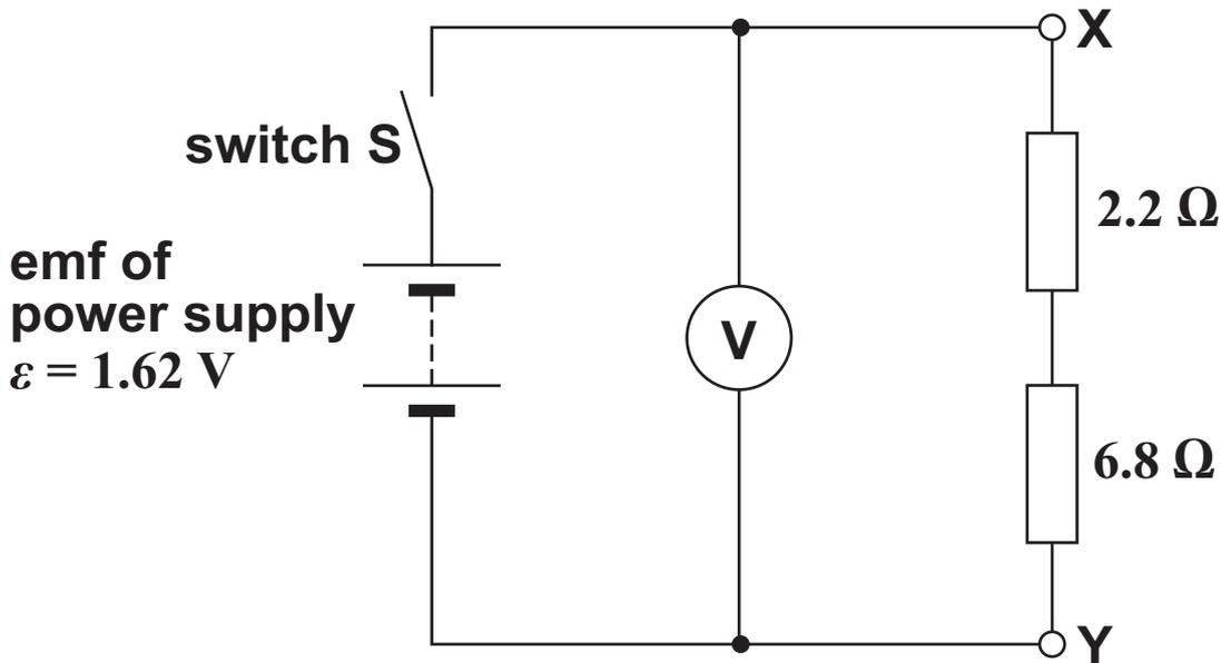
When  $S$  is closed the voltmeter reading  $V$  is  $1.14 \text{ V}$ .
