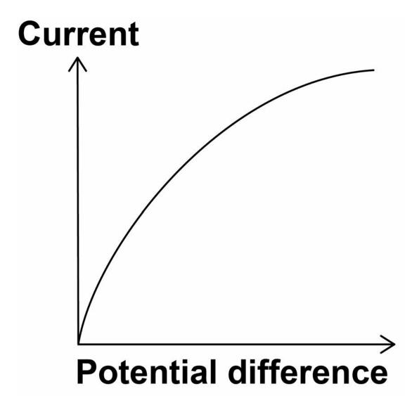
Explain how the resistance of a filament lamp changes as the potential difference across it increases. [3 marks]
