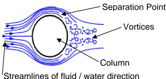
Fluid will flow around the column, separate and develop a vortex wake ( vortex shedding ) behind / downstream of the column.
