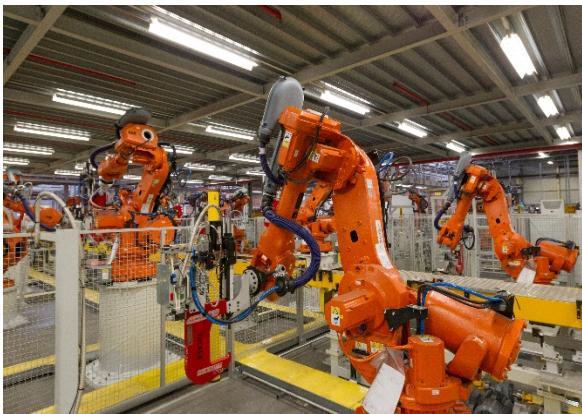
Many of the production line solutions developed and implemented by the Automated Technology Group are centred around the concept of a robot cell. This is a self-contained production cell which contains an industrial robot, and the associated ancillaries and safety equipment to enable the robot to perform its intended production operation.
