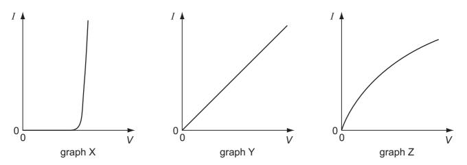
The components are a metal wire at constant temperature, a semiconductor diode and a filament lamp.
