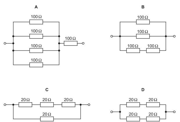
**37** Which circuit has a resistance of  $40\Omega$  between the terminals?
