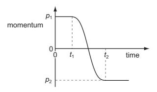
Initially, the momentum is  $p_1$  at time  $t_1$ . At time  $t_2$  the momentum is  $p_2$ .
