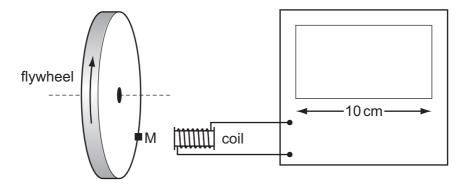
The flywheel has a small magnet M mounted on it. Each time the magnet passes the coil, a voltage pulse is generated, which is passed to the c.r.o. The display of the c.r.o. is 10 cm wide. The flywheel is rotating at a rate of about 3000 revolutions per minute.
