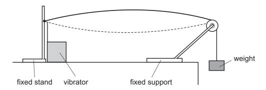
A vibrator is attached to the wire near the clamped end. A stationary wave with one loop is produced. The frequency of the vibrator is *f*.
