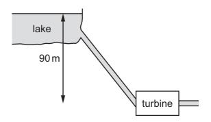
The mass flow rate of the water is 2400 kg min<sup>-1</sup>. The turbine has an efficiency of 75%.
