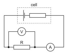
A student records the ammeter and voltmeter readings. She then connects a second identical external resistor in parallel with the first external resistor.
