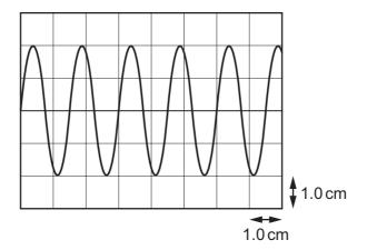
The time-base setting is 2.5 ms cm<sup>-1</sup> and the Y-gain is 2.0 V cm<sup>-1</sup>.
