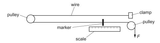
The wire passes from a clamp, around a frictionless pulley, and then to a second frictionless pulley where loads F are applied to it. A marker is attached to the wire so that the total length of wire between the clamp and the marker is initially 3.70 m. A scale is fixed near to this marker.
