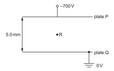
What is the magnitude and direction of the electric field at point R?
