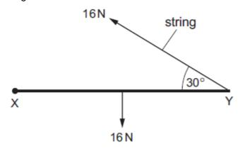
What is the horizontal component of the force acting at X?
