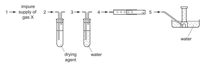
In which order should pieces of apparatus be joined together to collect a pure, dry sample of X?
