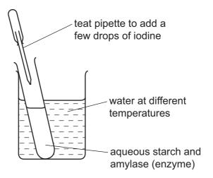
The experiment is set up as in the diagram and the time measured for the mixture to change from blue-black to colourless. The experiment is repeated at different temperatures. Typical results of this experiment are given in the table below.
