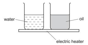
The temperature of the water and the temperature of the oil increase steadily. The increase in temperature of the oil is much greater than that of the water.
