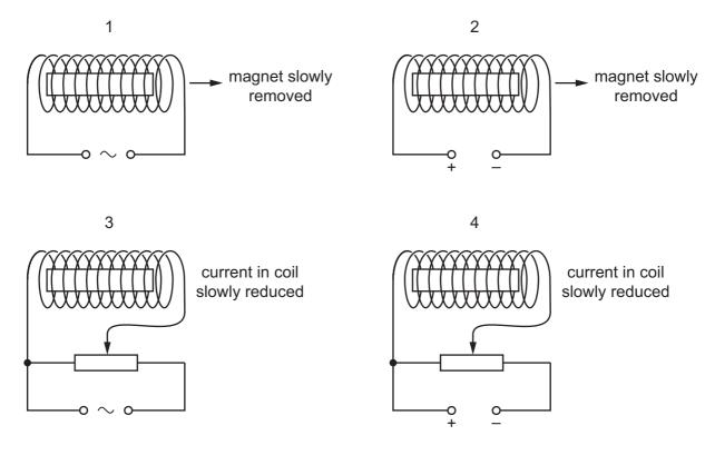
In which experiments is the magnet demagnetised?
