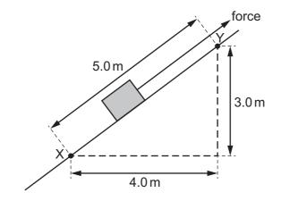
How much work is done against gravity in moving the box from X to Y?
