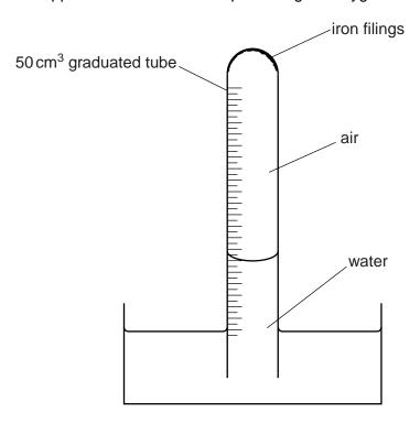
The iron filings react with oxygen, removing it from the air in the graduated tube.
