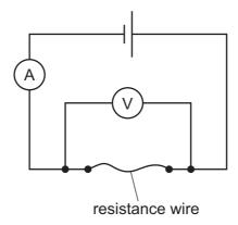
Which equation is used to calculate the resistance of the wire?
