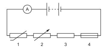
Which component causes the ammeter reading to increase when the temperature increases?
