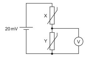
The cell has electromotive force (e.m.f.) 20 mV and negligible internal resistance.
