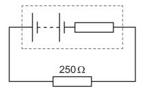
The current in the resistor is 40 mA for a time of 60 s. During this time 6.0 J of energy is dissipated by the internal resistance.
