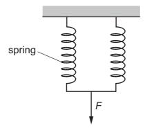
What is the extension and total elastic potential energy of this arrangement when the same force F is applied?
