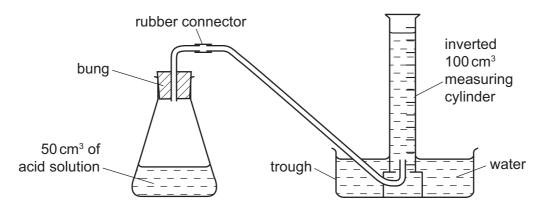
Using a measuring cylinder,  $50 \text{ cm}^3$  of acid **X** was poured into the conical flask. 0.5g of magnesium ribbon was added to the conical flask and the bung replaced.
