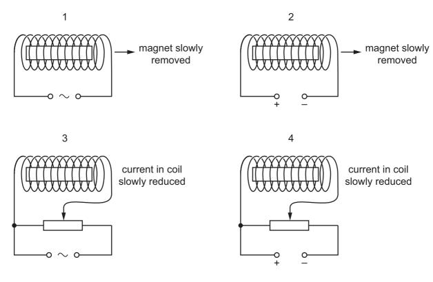
In which experiments is the magnet demagnetised?
