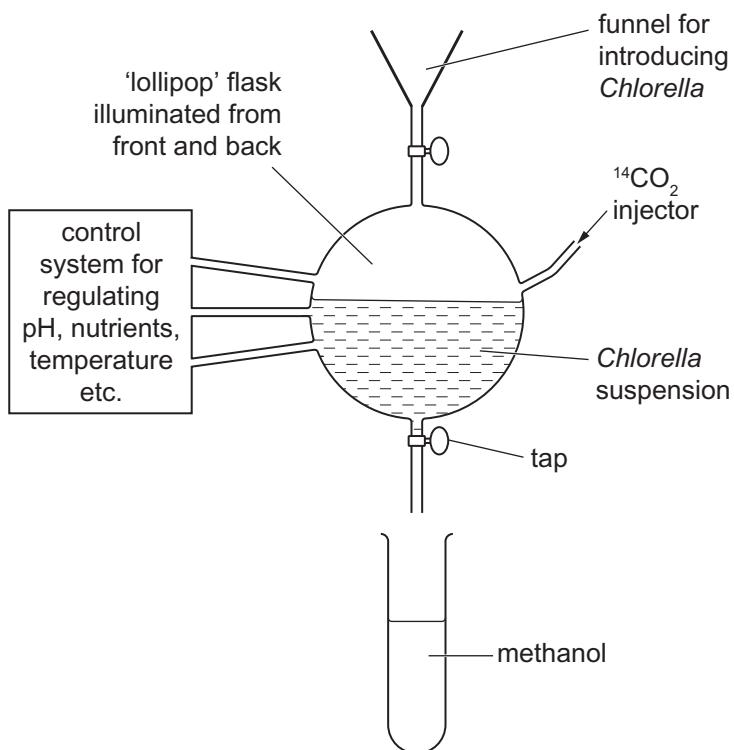
Calvin added radioactive carbon dioxide ( $^{14}\text{CO}_2$ ) to the apparatus and, after a very short period of time, he opened the tap to release the *Chlorella* (an autotrophic prototistian) into the methanol. This killed the *Chlorella* immediately and stopped any further reactions. The *Chlorella* was homogenised and the compounds present were identified by chromatography.
