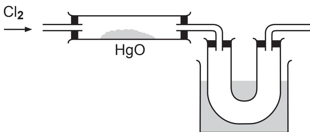
The escaping gases are passed through a U-tube which is cooled to –30°C.
