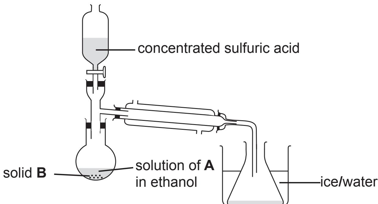
The acid from the dropping funnel is added slowly. As the reaction proceeds and the solution in the round-bottom flask boils, a colourless liquid is collected in the conical flask.
