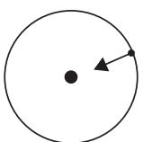
$\frac{GMm_1}{d^2} = m_1 d\omega^2$ $\omega^2 = \frac{GM}{d^3}$ $T = \frac{2\pi}{\omega}$ $= 2\pi \sqrt{\frac{d^3}{GM}}$ $= 2\pi M^{-\frac{1}{2}} d^{\frac{3}{2}} G^{-\frac{1}{2}}$ $\therefore k = 2\pi$ | M1 W1<br>W1<br>M1<br>W1 |
