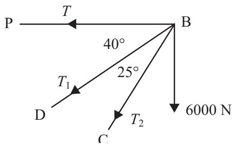
↖ :  $T \times \sin 40^\circ = T_2 \times \sin 25^\circ + 6000 \times \sin 50^\circ$
