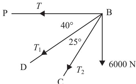
Horizontally:  $T + T_1 \cos 40^\circ + T_2 \cos 65^\circ = 0$  (1) M1 W1
