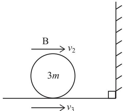
$$v_3 = -ev_2 = -e(v_1 + eu)$$
