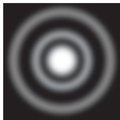
Electron diffraction rings seen on the fluorescent screen
