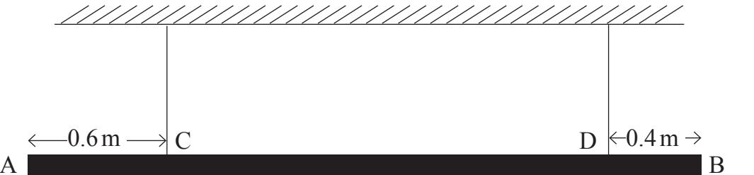
A mass of 6 kg is attached to the rod at the end A and a mass of 8 kg is attached to the rod at the end B.
