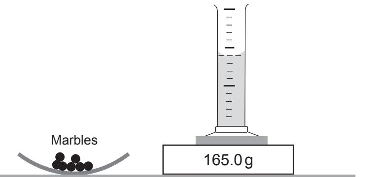
The measuring cylinder was partly filled with water and then placed on the electronic scales. Marbles were added to the cylinder. The measurements taken by the student are shown below.
