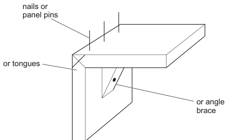
Normally they are nailed with panel pins or it can be strengthened with glue blocks, or angle braces or tongues.
