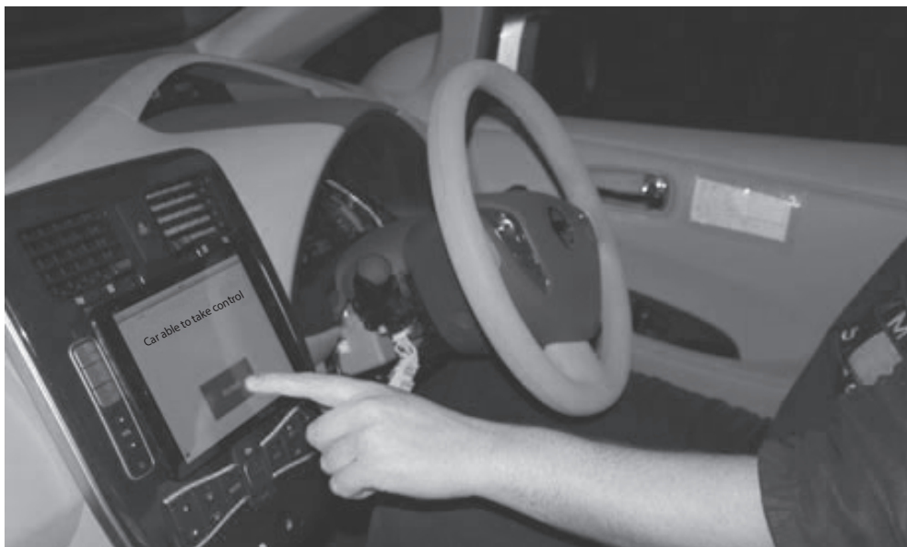
Figure 4: Control panel of a self-driving car
