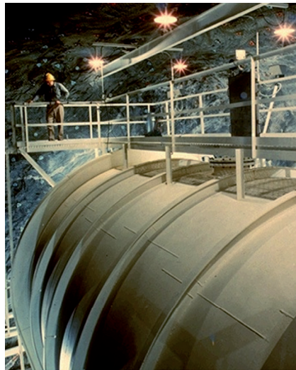
Figure 2: The Homestake solar neutrino detector
