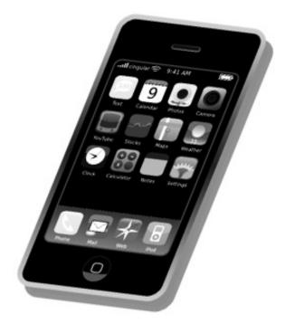
The iPhone 4 includes a panel laminated on the glass which uses electrical fields to sense the user's touch. It has a multi-touch feature that can register simultaneous touches. The user can bring up different information or menus by actions such as swiping, tapping and pinching. Information is displayed on the panel using a "Retina display".
