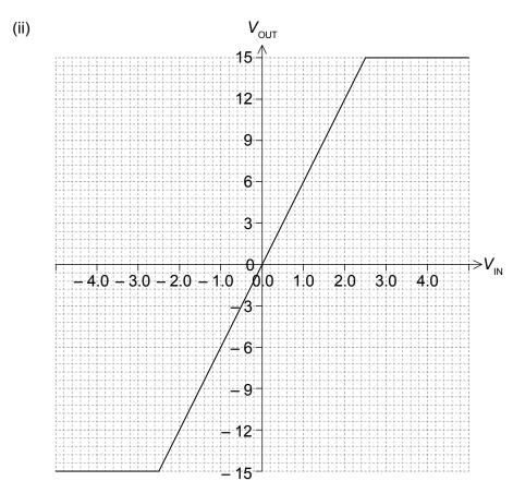
general shape of graph correct; straight line between –2.5 V and 2.5 V; plateau at –15 V and +15 V beyond this;
