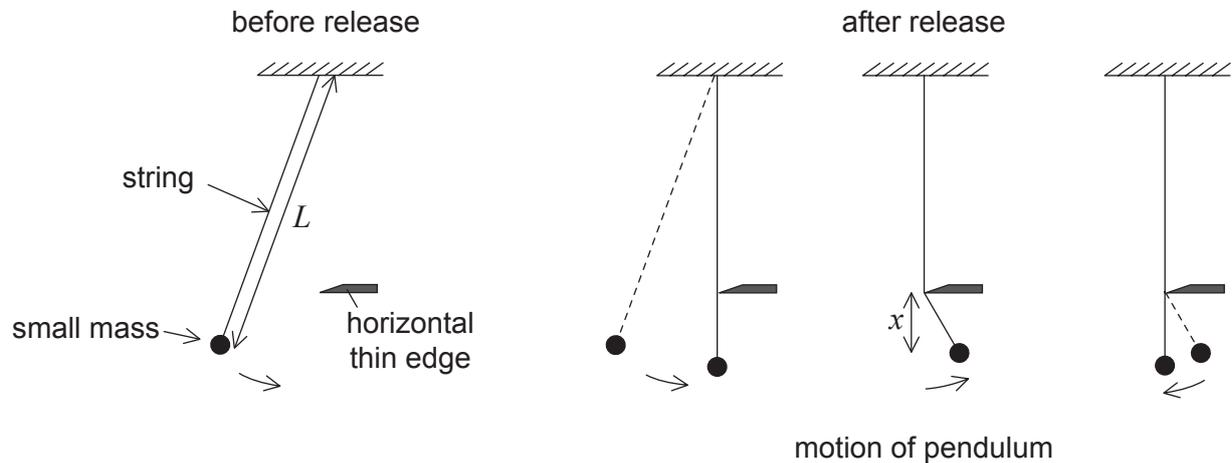
The length  $L$  of the string is kept constant during the experiment. The vertical position of the horizontal thin edge is varied to change  $x$ .
