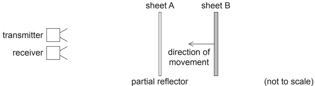
Sheet A is fixed and sheet B is moved towards it. While sheet B is moving, the intensity of the signal detected at the receiver goes through a series of maximum and minimum values.
