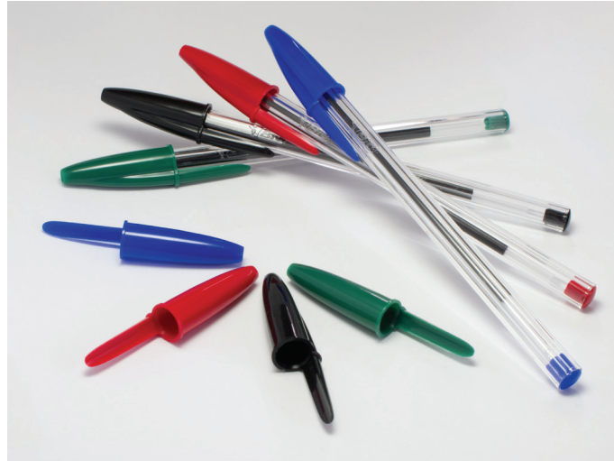
Figure 1: Ballpoint pens produced by injection moulding
