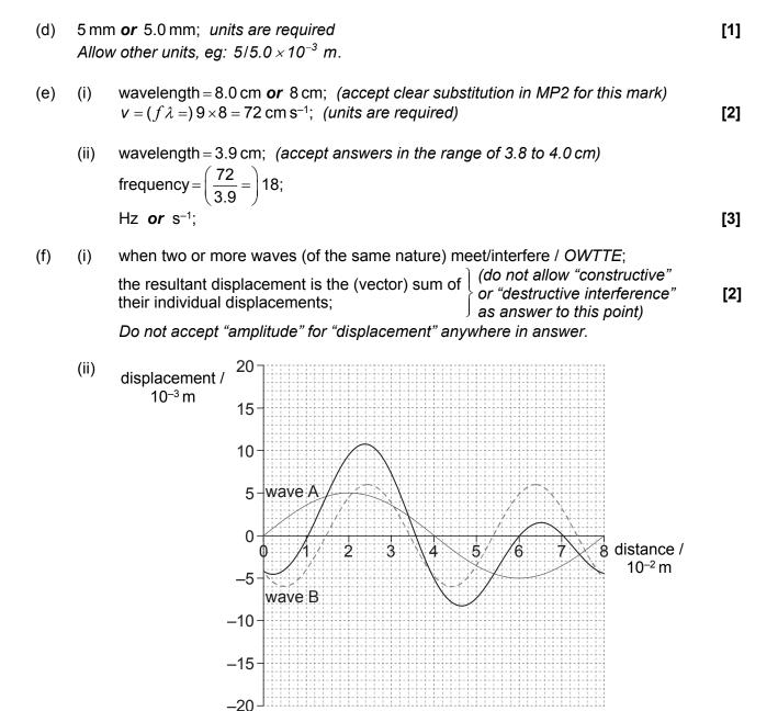
start and end points correct (equal B) and crossing points on distance axis correct (1, 3.6, 6, 7); peaks and troughs at (2.4, 11) (4.6, -8) (6.5, 1.5);
