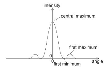
According to the Rayleigh criterion, when the diffraction patterns of two slits are just resolved
