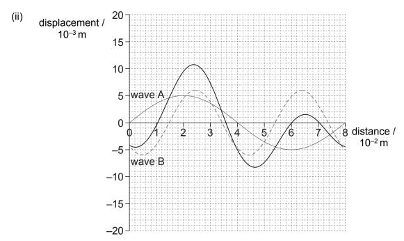
start and end points correct (equal B) and crossing points on distance axis correct (1, 3.6, 6, 7); peaks and troughs at (2.4, 11) (4.6, -8) (6.5, 1.5);
