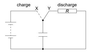
What is the nature of the current and magnitude of the initial current in the resistor after the switch is connected to terminal Y?
