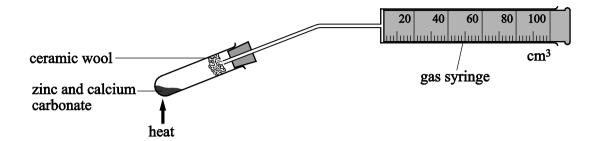
A mixture containing 0.27 g of powdered zinc and 0.38 g of powdered CaCO<sub>3</sub> was heated strongly for two minutes. The volume of gas collected in the 100 cm<sup>3</sup> syringe was then measured. The experiment was then repeated.
