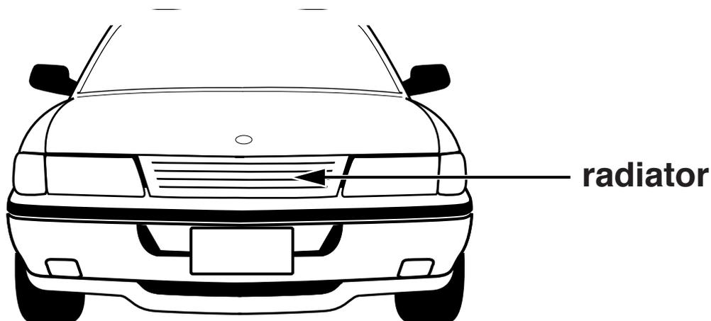
**Hot water from the engine gives out heat in the radiator to keep the engine cool.**
