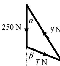
$\frac{S}{\sin 145^\circ} = \frac{T}{\sin 8.5^\circ} = \frac{250}{\sin 26.5^\circ}$ $S = 321.4$ $T = 82.8$ | <p>M1</p> <p>M1</p> <p>A1</p> <p>A1</p> | <p>Either Drawing and using a triangle of forces</p> <p>Or Quoting and using Lami's Theorem</p> <p>Correct form of these equations</p> <p>CAO</p> <p>CAO</p> |
