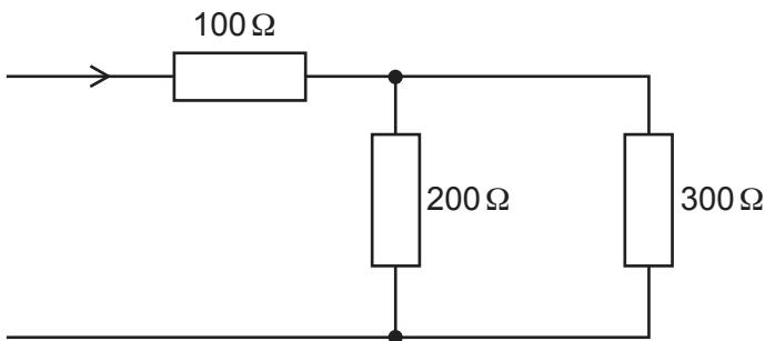
The resistance of each resistor is shown.
