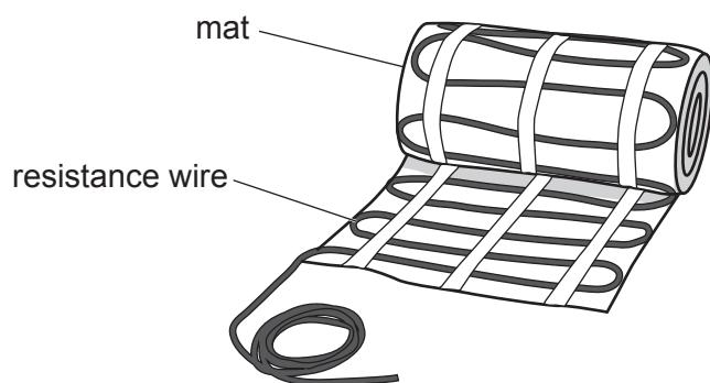
Each mat has resistance wire. The wire has cross-sectional area  $6.7 \times 10^{-8} \text{ m}^2$ , total length 25 m and resistance 180  $\Omega$ . Each mat dissipates 300 W when connected to the mains supply.
