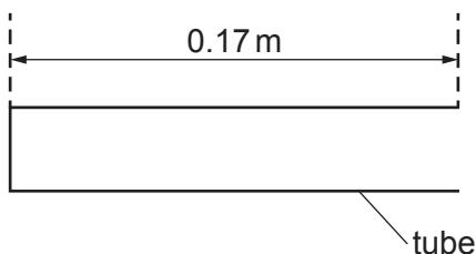
The length of the tube is 0.17 m. The speed of sound in air is  $340\text{ ms}^{-1}$ .
