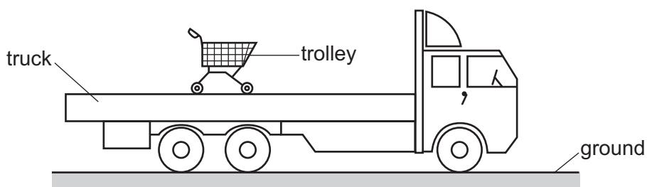
The truck suddenly accelerates. The trolley is observed to remain in the same position relative to the ground.
