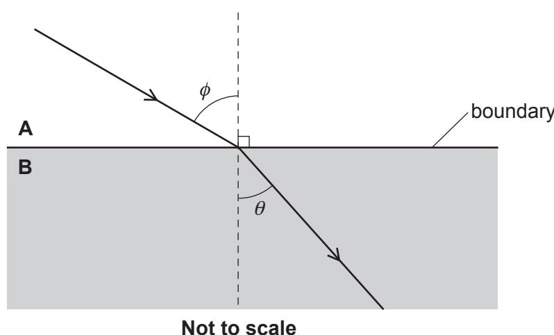
The refractive index of **B** is 1.3 times greater than the refractive index of **A**.
